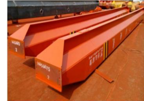
Crane main girder
