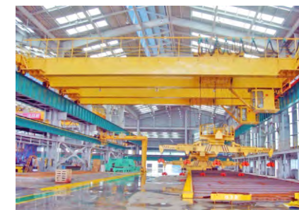
Electromagnetism bridge crane
