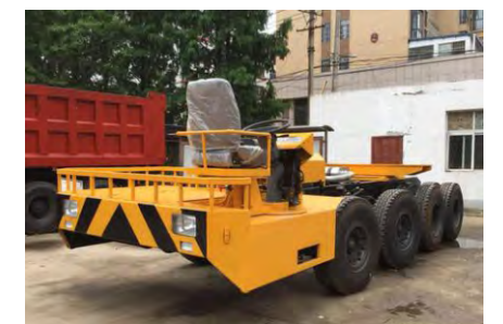
Girder transportation vehicle
