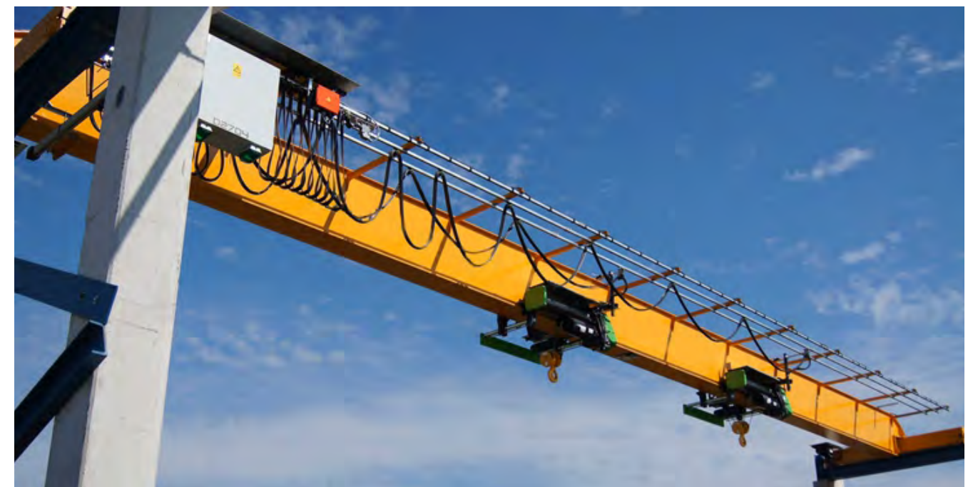
Single girder bridge crane
