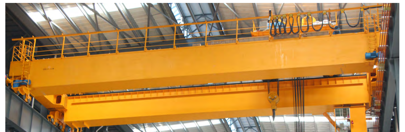
Double beam bridge crane
