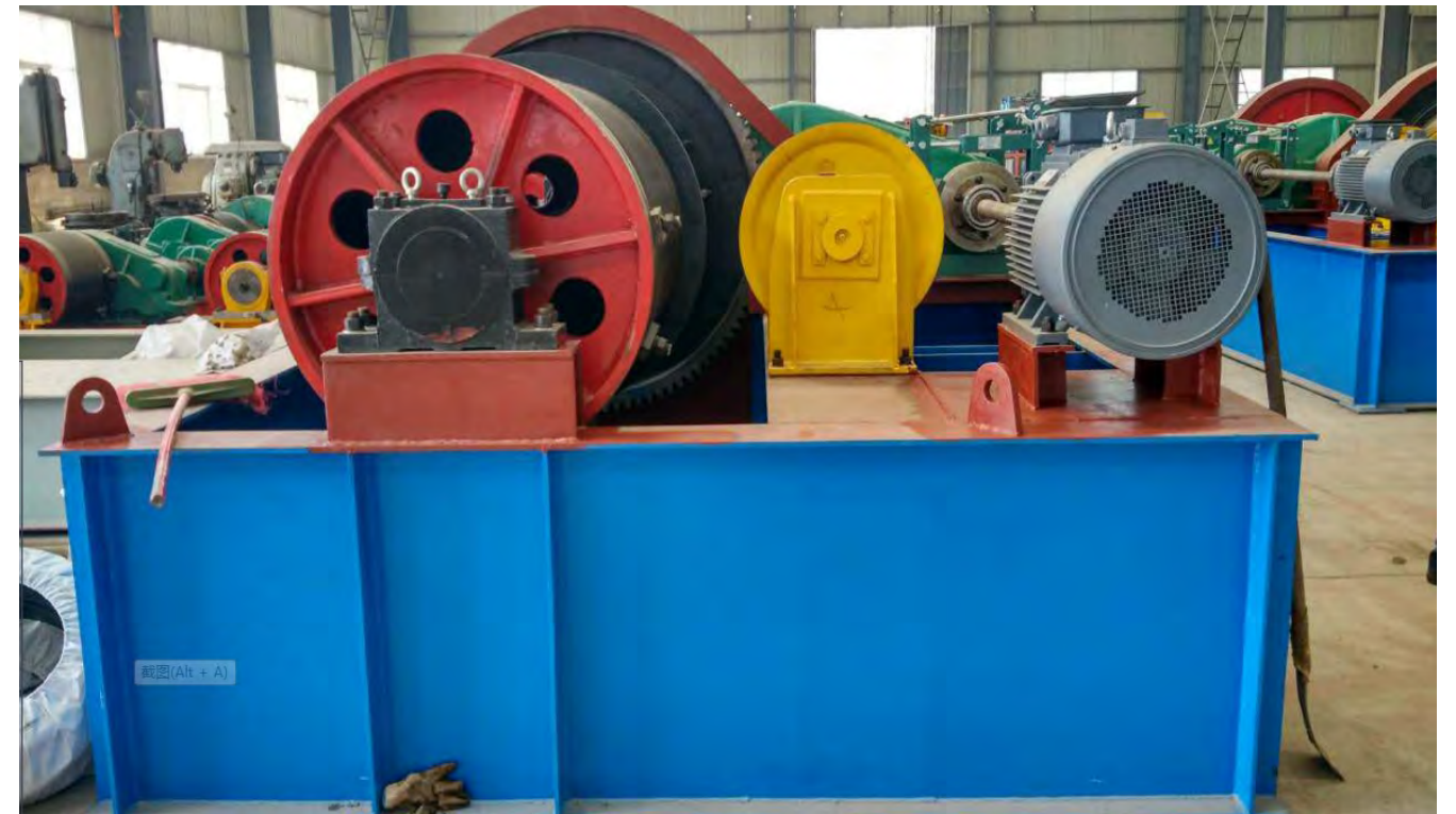
Winch trolley for gate hoist
